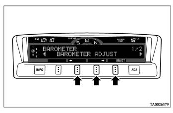
3. Adjust the barometer by pressing the function buttons.
