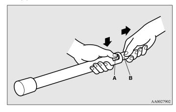
2. With the snap pin (C) pushed, insert the inside handle until it is locked
