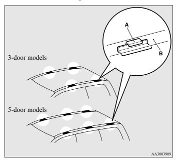
When installing the roof carrier, use the brackets (A). The brackets (A) are located under each roof drip moulding (B).
