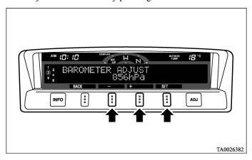
"+"- To adjust the barometer
