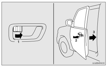
Set the inside lock knob (1) to the locked position, and while pulling the outside handle up (2), close the door (3).
