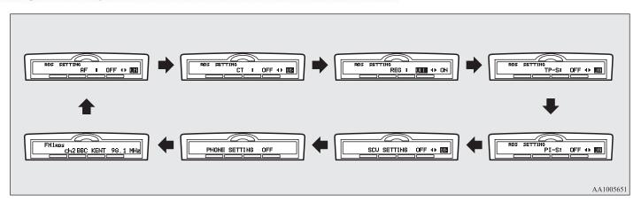
2. Press the "MENU" button (4) repeatedly to select the mode you wish to change. The order is: AF → CT → REG → TP-S → PI-S\* → SCV → PHONE → Function setup mode OFF.
