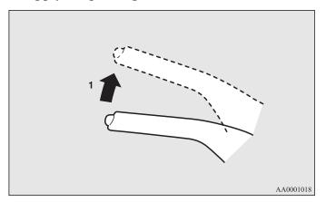
1- Pull the lever up without pushing the button at the end of hand grip.
