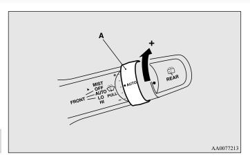
The wipers will operate once if the lever is moved to the "AUTO" position and knob (A) is turned in the "+" direction when the ignition switch is "ON" position.
