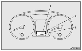
The service reminder shows the number of months (1) and driving distance (3) remaining until the next 12-monthly (15,000 km or 9,000 miles) inspection. When the next inspection is nearly due, the display shows "----". At this time, a spanner mark (2) is shown for a few seconds whenever the ignition switch is turned from the "OFF" position to the "ON" position.
