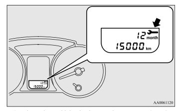
3. When the vehicle is inspected at a MITSUBISHI MOTORS Authorized Service Point, the number of months and driving distance remaining until the next inspection will be shown.
