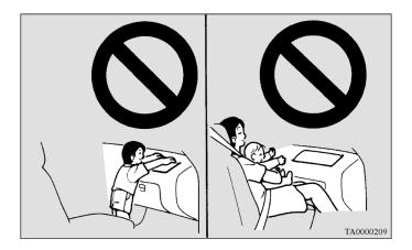
Use rearward facing child restraints in the rear seat or turn off the front passenger's airbag ON-OFF switch. (Refer to "To turn an airbag off" on page 2-64.)
