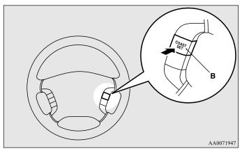
To slow down your speed in small amounts, press the "COAST SET" switch for less than about 1 second and release it. Each time you press the "COAST SET" switch, your vehicle will slow down by about 1.6 km/h (1 mph).
