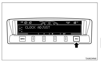
2. It is possible to adjust the clock using the function buttons
