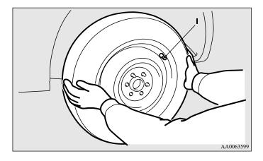
9. Temporarily tighten the wheel nuts (flange nuts) until their flange section comes in contact with the wheel and it is no longer loose.
