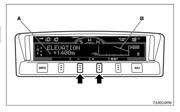
'+"- Adjustment of elevation
