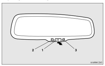
Normally, use the automatic mode. When the switch (1) is pressed, the indicator (2) illuminates and the reflection factor of the mirror is automatically changed.
