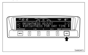
2. Press the "←" or "→" function button to select the setting you wish to adjust (daytime or nighttime). Then press the "SELECT" function button.
