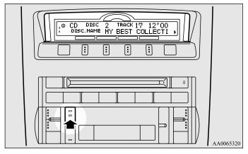
Push the CD button (4) if the discs are already in the autochanger. The autochanger will enter CD mode and start playback. The disc number, the track number and the playing-time will appear on the display. The discs in the unit will be played consecutively and continuously.
