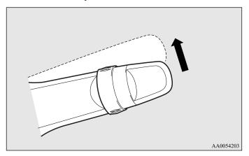
The wipers will operate once if the wiper lever is raised to the "MIST" position and released. This operation is useful when it is drizzling, etc. The wipers will continue to operate while the lever is held in the "MIST" position.
