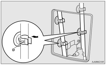
4. Reverse the removing procedure when storing the tool, jack and jack handle.
