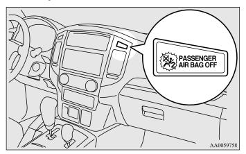
The indicator normally illuminates when the ignition switch is turned to the "ON" position, and goes off a few seconds later. When the front passenger's airbag ON-OFF switch is turned OFF, the indicator will stay on to show that the passenger front airbag is not operational.
