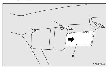
To block out a broader range of glare from your side, swing the sun visor sideways and pull out the slide plate (B).
