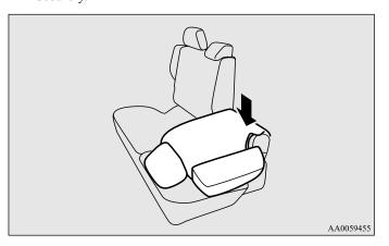
3. Raise the seatback until it locks securely into place. Push lightly on the seatback to confirm that it has actually been secured.
