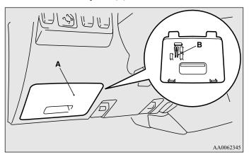
4. The replacement of fuses located in the driver's seat leg area should be performed from the hole of the fuse block lid.
