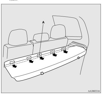
2. Raise the rear shelf, then pull it upward to remove it from the groove (B) on each side of the luggage area.
