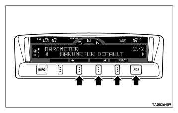
2. Press the "SET" function button. The display will flash twice and the barometer indication will return to the factory setting.
