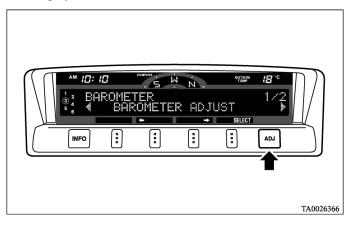
2. Press the "←" or "→" function button to select the "BAROMETER ADJUST" display. Then press the "SELECT" function button.
