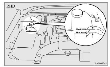
If the level is below the "MIN" mark, check according to the following procedure:
