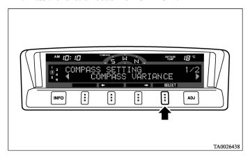
2. Press the function button for "←" or " → " to set the desired declination.
