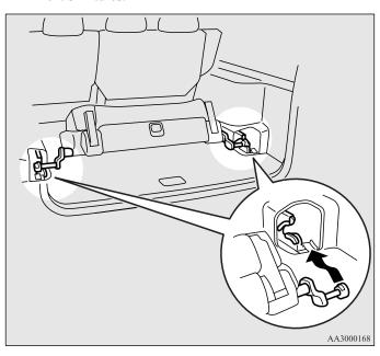
2. Confirm that the seat's mounting arms are secured by the hooks (A).
