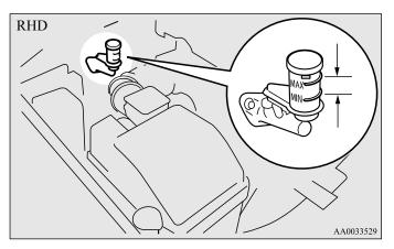
If the fluid level falls markedly in a short length of time, it indicates leaks from the clutch system.
