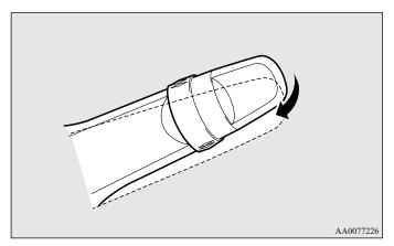
With the ignition switch in the "ON" position, if the lever is moved to the AUTO position and pulled towards you a little, the wipers operate once.
