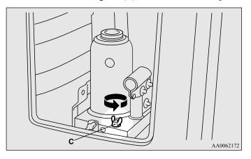
3. Remove the tool and the jack handle from the holder (D), and take it out.
