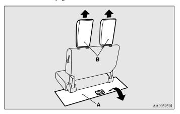
2. Stow the removed head restraints in the luggage floor box with their front faces facing upward.
