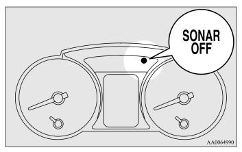
To have the system operating again, push the "SONAR" switch again. When the system is operating again, the buzzer sounds once and the "SONAR OFF" indication lamp turns off.
