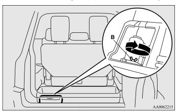
6. Reverse the removing procedure when storing the tool, jack and jack handle.
