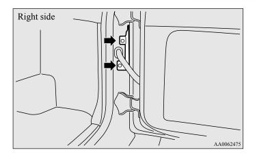
3. Remove the socket and bulb assemblies by turning it anticlockwise.
