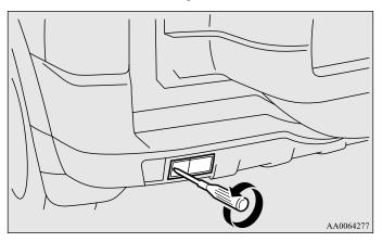
2. Remove the socket and bulb assembly together by turning it anticlockwise, and then remove the bulb by pulling it out.
