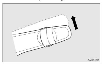
The wipers will operate once if the lever is raised to the "MIST" position and released when the ignition switch is in the "ON" or "ACC" position. The wipers will continue to operate while the lever is held in the "MIST" position.
